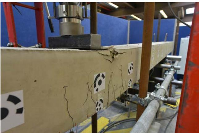
**Figure 1.** Bending failure of laboratory beam
