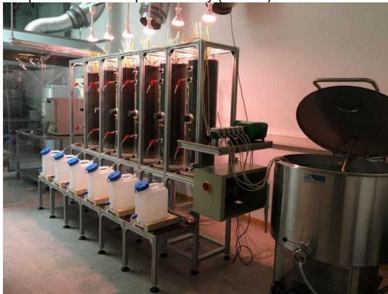
Once selected the most promising adsorbing material, an intermediate test will be performed in the treatment plant of Reisdorf, Luxembourg (i.e. 4000 PE) in order to see the effect of real matrix. The knowledge gained from these lab scale studies together will be then used to design and dimension a full scale wetland to be installed in the WWTP of Echternach, Luxembourg (i.e. 20000 PE) and subsequently for decision policy support in the Greater Region.
