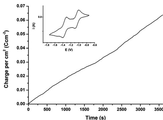
Fig. 1 Total charge per cm<sup>2</sup> passed during a 60 minute (3600 s) deposition holding the voltage at 0.30 V. Inset: cyclic voltammogram of BuPTCDI between -1.0 and 0 V in 0.1 M TBABF<sub>4</sub> in THF.
