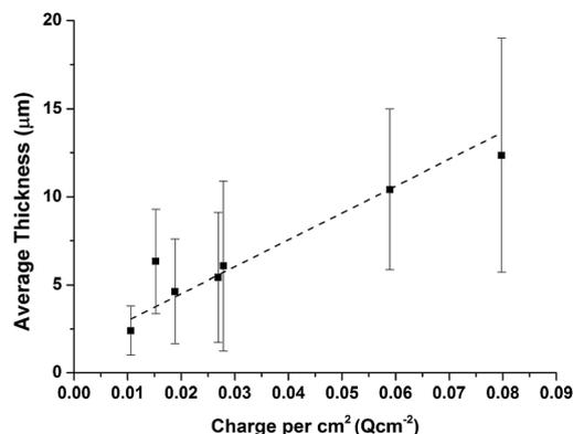
Fig. 4 Average film thickness versus charge per  $\text{cm}^2$  passed. The bars represent maximum and minimum thicknesses observed across the film.
