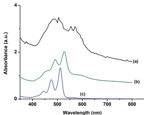
Fig. 6 UV/Vis spectra of BuPTCDI (a) electrodeposited on FTO, (b) dissolved in DMSO and (c) dissolved in THF.
