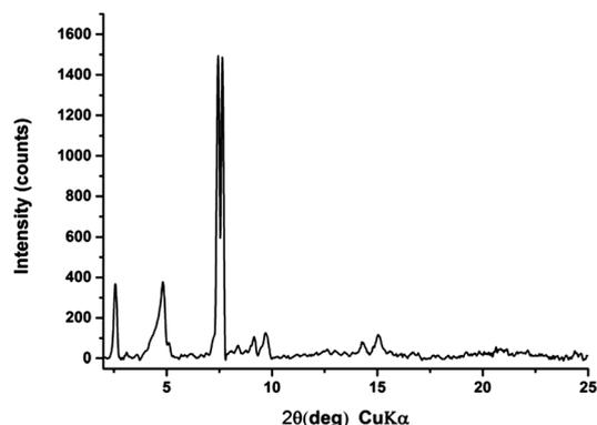
Fig. 5 XRD pattern of an electrodeposited BuPTCDI film.
