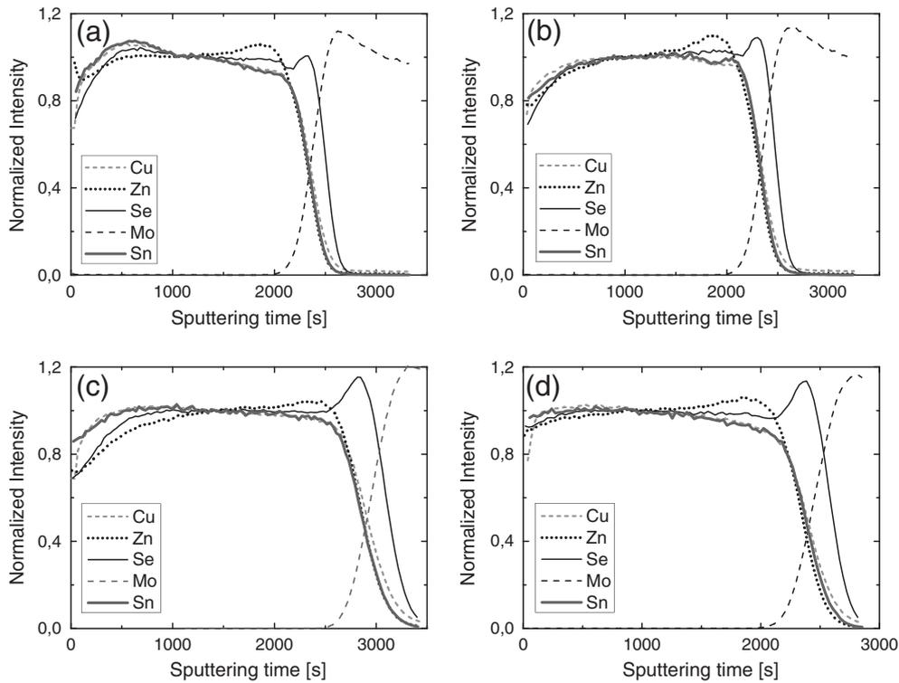
Fig. 4. Different SIMS depth profiles for two different absorbers I and II: (a) absorber I without etching, (b) absorber I after HCl etching, (c) absorber II without etching, and (d) absorber II after Br<sub>2</sub>-MeOH etching.
