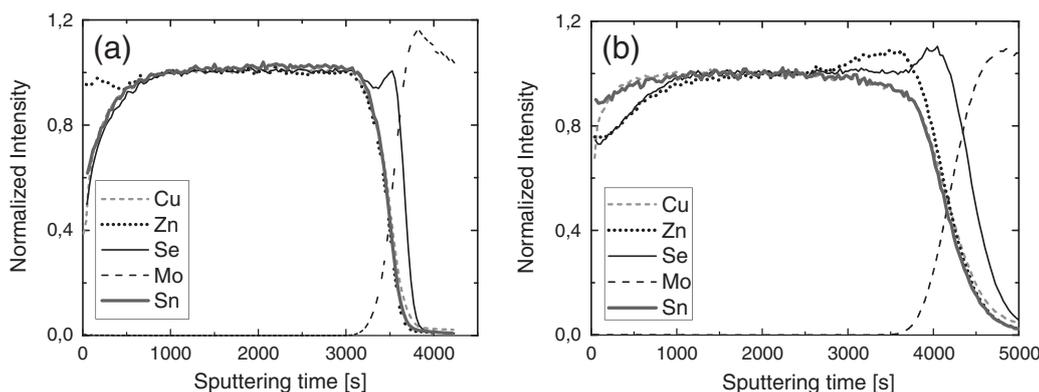
Fig. 2. Two SIMS depth profiles of unetched absorbers for (a) absorber that gave a solar cell efficiency higher than 4% and (b) absorber that gave no working solar cell.
