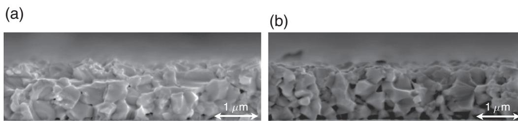
Fig. 3. SEM cross-sections of sample I (a) without etching and (b) after 1 min HCl etching.
